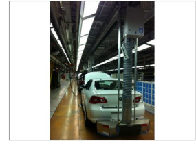
上海大众三厂2线（半自动滑轨式软管尾气抽排系统） SVW CP3 2nd line ( Half-Automatic oval System with conveyor)
